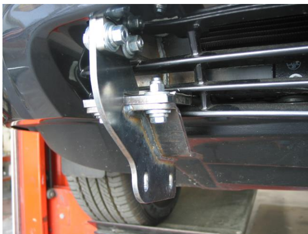
Figure 5: External mounts fitted with protection bar removed for photo. NOTE lower nut and washer combination.
